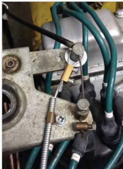
Pic 2: Cable attachment to bonnet catch.
